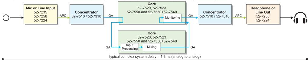
**Input Processing, typical:** subsonic filter, 4 band EQ, compressor, limiter (Note: the delay is constant and independent of the number of functions inside the processing chain)
