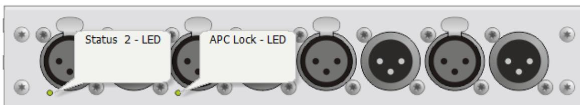
Positions of Status 2 - LED and APC Lock - LED on 52/XC I/O module front panels. Shown example: 52-7111
