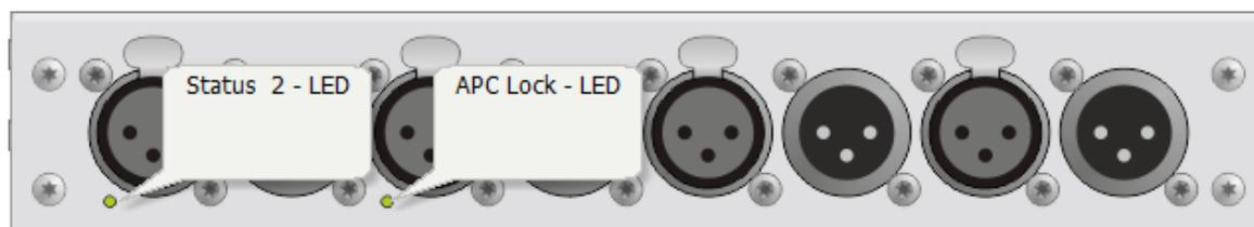
Positions of Status 2 LED and APC Lock LED on 52/XC I/O module front panels.
