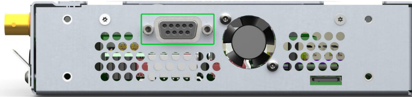
52-7424 XC2 Core - side view with one male DSub-9 serial RS232 port
